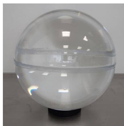
Figure 20. Sphere of ultrapure water used for proton reference.
